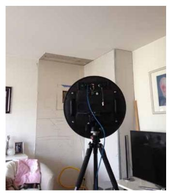
tions. The camera could be set up on the tripod, but also positioned on the floor, in a bed, on a couch or just hold it by hand all based on what part of the room one would like to listen to and get the acoustic image from. The 40 cm camera proved to be very handy in a measurement situation where it was not given beforehand exactly where the source of interest was positioned. In that way the camera could easily be used to scan around different parts of different rooms.
