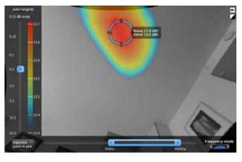
In addition to measurements in the living room subsecuent measurements were also made in the two bedrooms. These measurements displayed the same result, the energy of the noise did not come from the walls, but were confined to the roof. All in all this was a very strong indication that the problem was piping located in separating floors between apartments.
